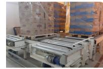
We just commissioned a material handling project in a major food plant, comprising of 2 levels of pallet conveyors in a loop layout with lifting tables for diverting, and a pallet lift between the two levels.
